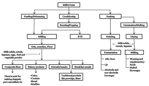
Schematic diagram for developing millet-based composite foods\
